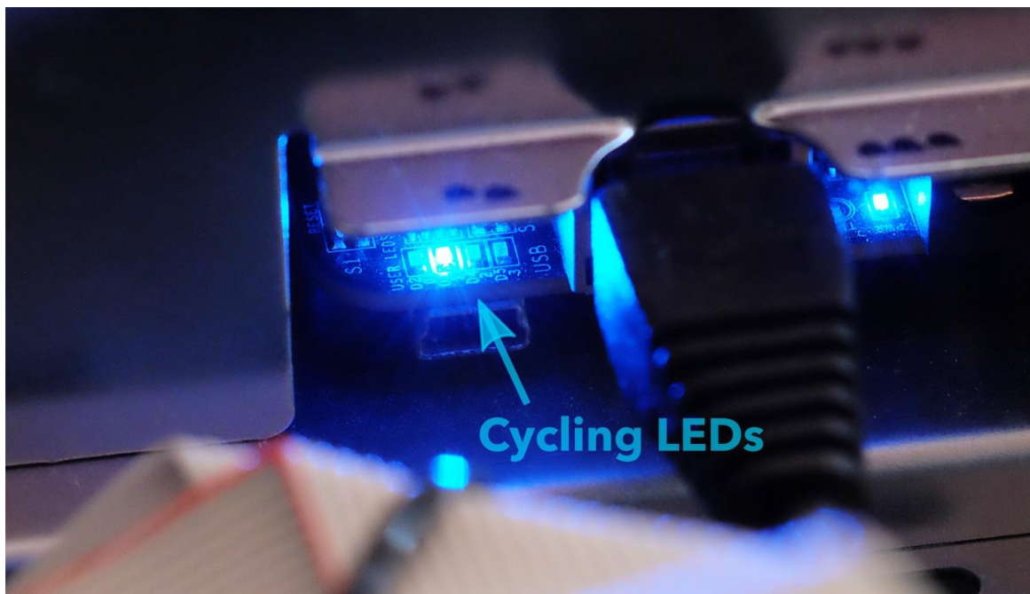
Photo 4. LEDs cycle while upgrade is in progress
